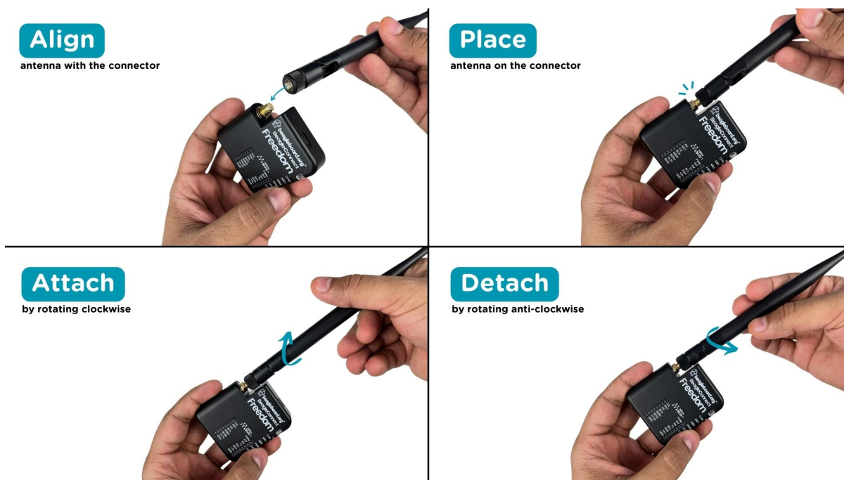
Fig. 2.2: Attaching antenna to BeagleConnect Freedom
