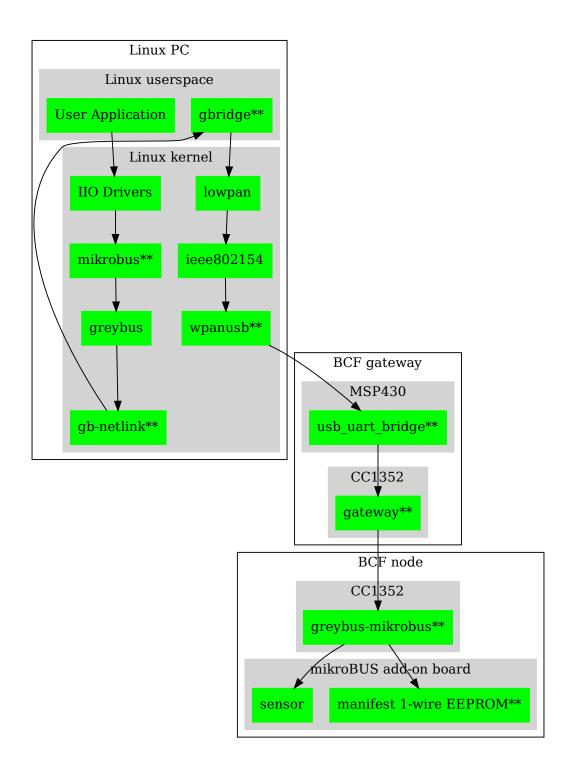
Fig. 3.1: BeagleConnect Software Architecture Diagram
