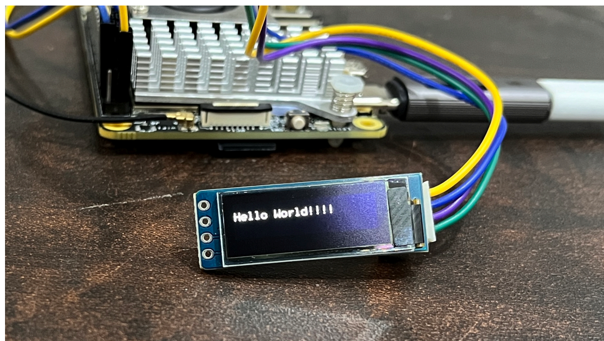
Fig. 5.22: Hello World!!!! on 128x32 OLED
