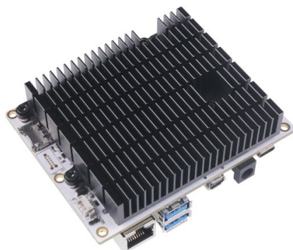
Fig. 6.10: BeagleBone AI-64 back with heatsink at 45° angle
