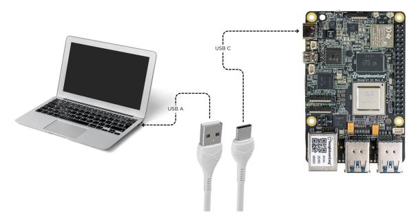
After connecting, you should see the power LED glow, and soon just like with other Beagles, you'll see a virtual wired connection on your computer. To access the board you can use SSH as shown below.
