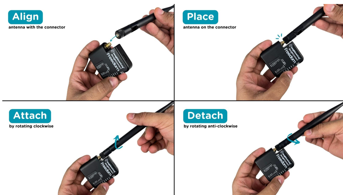
Fig. 2.2: Attaching antenna to BeagleConnect Freedom
