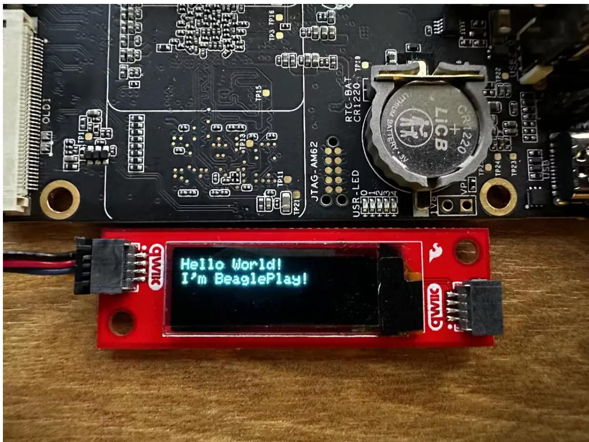
Fig. 5.17: BeaglePlay QWIIC OLED HelloWorld.py Output
